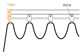
Item FF3664 holds the cable in position and function as endstop for the cable carriages.
