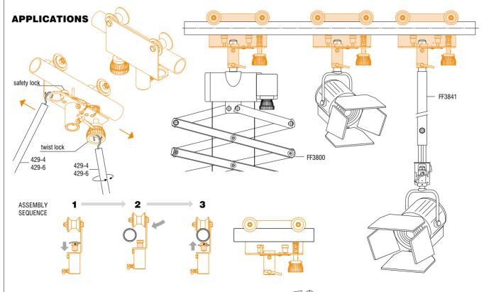
Metric measurements should be taken as reference. Imperial values have been calculated from metric and rounded to nearest 1/32 inch. EAC IMPORTANT: installation must be carried out by qualified personnel and in accordance with the safety regulations of the country/region of installation.
