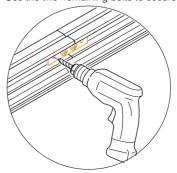
IMPORTANT: Don't place the alignment connectors in the lower section of the rail where the carriages run.
