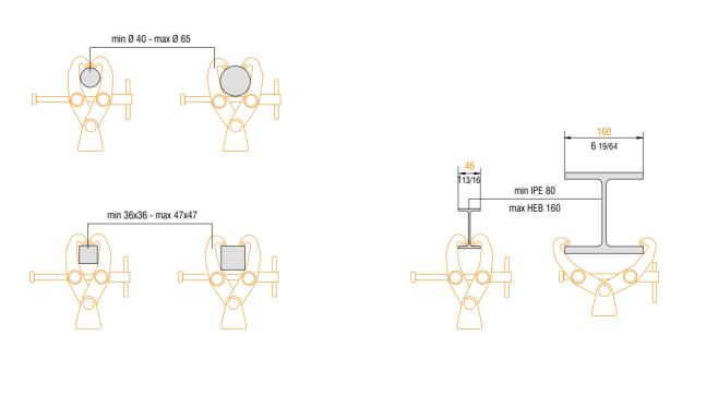
**CLAMPS**  Metric measurements should be taken as reference. Imperial values have been calculated from metric and rounded to nearest 1/32 inch. IMPORTANT: installation must be carried out by qualified personnel and in accordance with the safety regulations of the country/region of installation.
