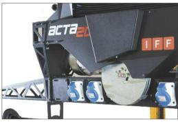
Any type of electrical socket can be supplied (32A IEC309, 16A IEC309, Schuko, BS 1363, DMX, Audio)
