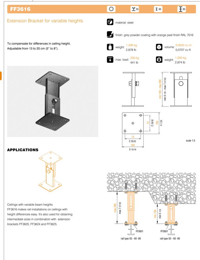
Metric measurements should be taken as reference. Imperial values have been calculated from metric and rounded to nearest 1/32 inch. EA DMPORTANT: installation must be carried out by qualified personnel and in accordance with the safety regulations of the country/region of installation.
