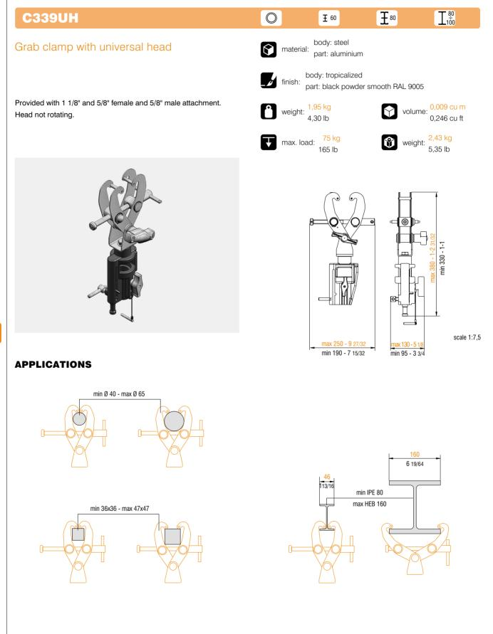
Metric measurements should be taken as reference. Imperial values have been calculated from metric and rounded to nearest 1/32 inch. EI () IMPORTANT: installation must be carried out by qualified personnel and in accordance with the safety regulations of the country/region of installation.
